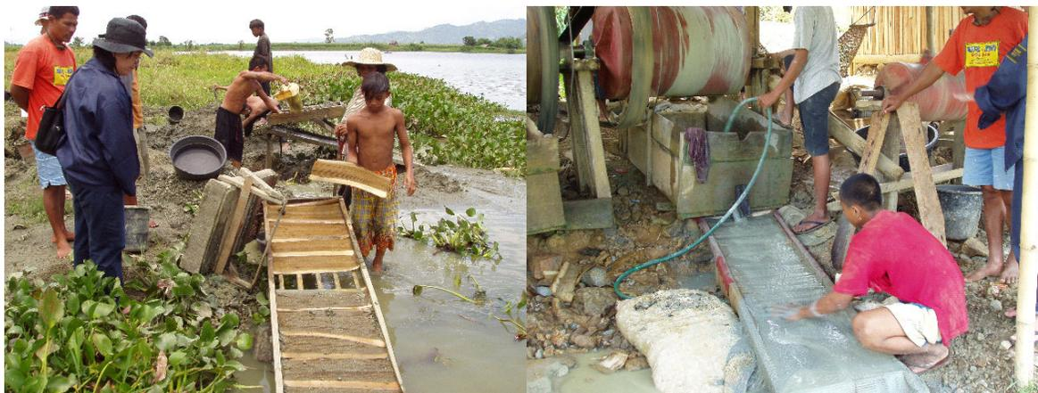
**Figure 37.** Family-based (left) and mechanized (right) gold panning operations along Kalinawan River.
