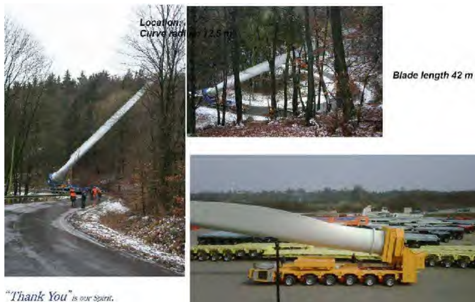
Figure 4-4-19: An Example of a Special Standing Transport Vehicle
