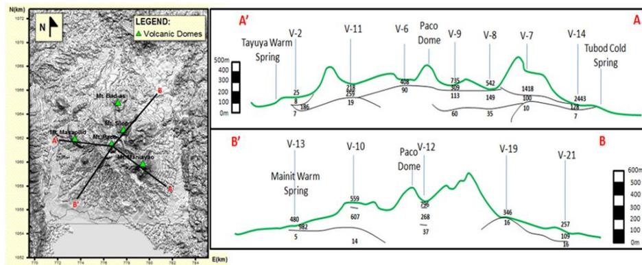
**Figure 3: Resistivity cross sections from the Schlumberger vertical electrical soundings (VES) along two intersecting profile lines within PMVC (modified from Catane et al., 1989). Subsurface resistivity values are in ohm-m.**
