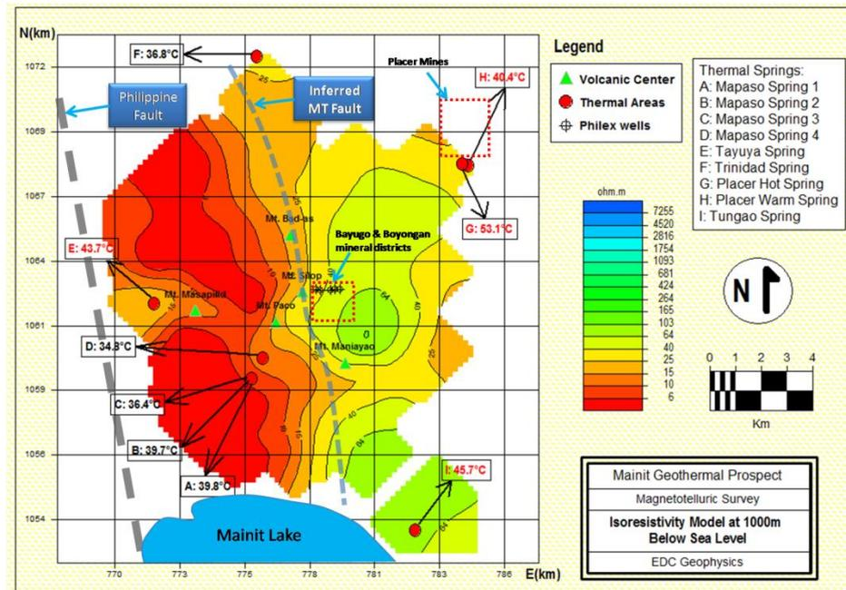
**Figure 6: Isoresistivity map at 1000m below sea level showing the location of the Volcanic Domes, the Philippine Fault, the inferred MT fault which was interpreted from the MT resistivity gradient, thermal springs and their surface temperatures. Mining districts in Bayugo, Boyongan and Placer are also included.**
