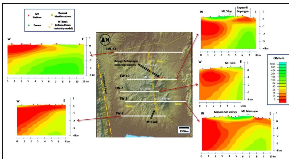
**Figure 4: Major 2D resistivity sections of the Mainit Geothermal Prospect showing the inferred MT fault.**
