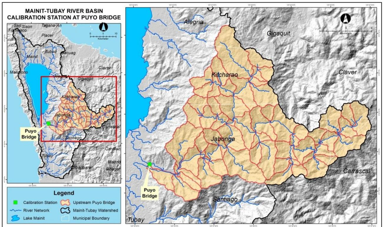
Figure 5. Mainit-Tubay River basin and the upstream sub-basins of the Puyo Bridge calibration station.
