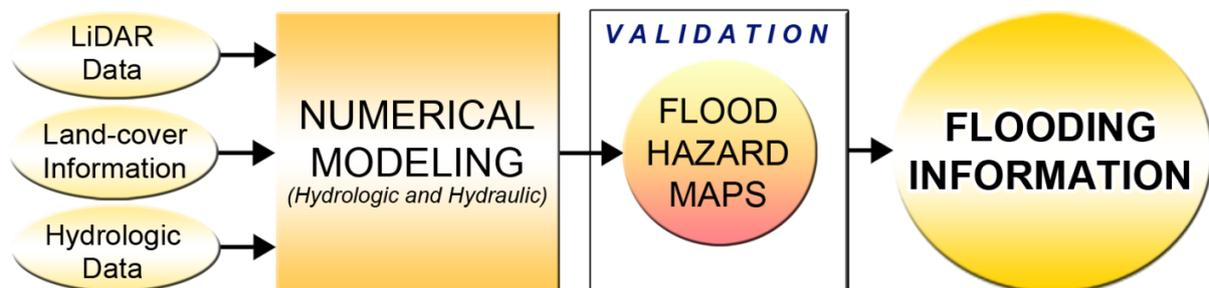
Figure 2. The flood hazard map generation process.
