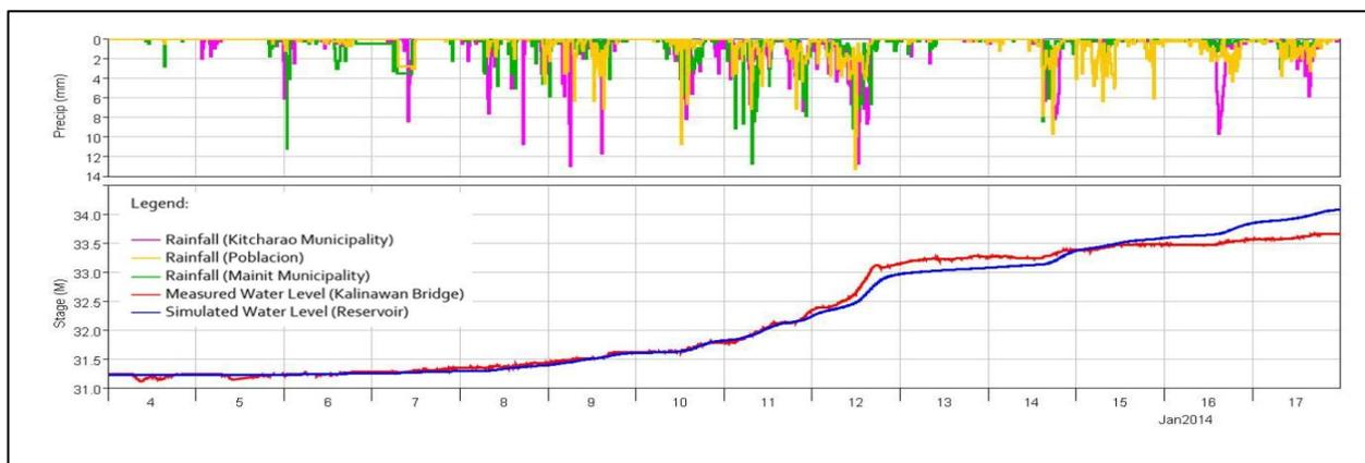
Figure 9. Graph showing the comparison between the edited stage readings at Kalinawan Bridge water level station and the simulated stage readings at the lake of the preliminary Mainit-Tubay HEC HMS model.
