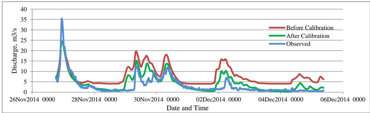
Figure 10. Comparison between the simulated discharge before and after calibration of the HEC HMS model.
